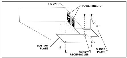
Figure 4.1: IPS-800 Series Cable Keeper Installation
